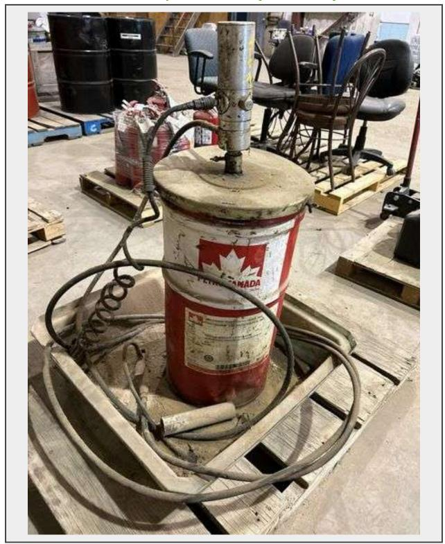
Notes Pneumatic Grease Pump with Precision Synthetic Heavy 460 (partial can)
