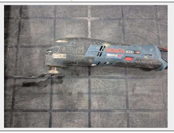
**Notes** 1 Bosch Cordless Ossilating Cutoff Tool (Comes with 2 Batteries, 1 Battery Charger, 4 Attachments and an Allen Key Wrench).
