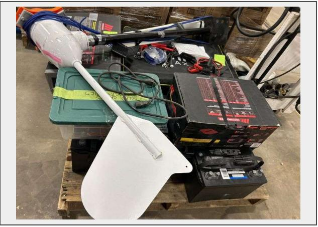
**Notes** 500 watts of folding solar panels with cases. 800 watt turbine with 25' #10 cable. 6 Deep cell batteries. 120 AMPH of storage. (2) 3000 watt power inverter's. (One sine wave the other modified wave)
