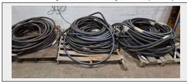
Notes 3 Pallets of High Pressure Water Blasting Static Hoses (14500 PSI)
