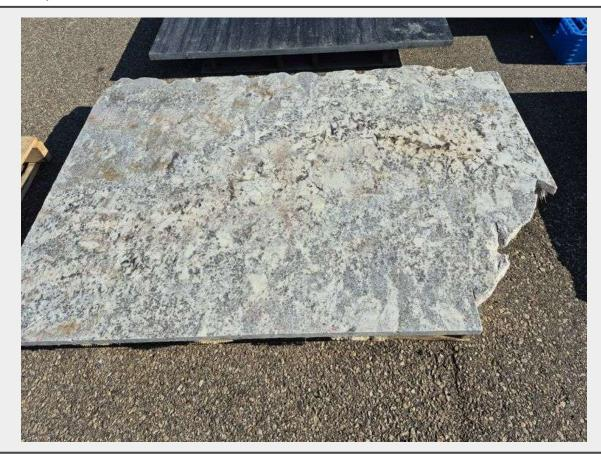
**Notes** 1 Slab of Granite irregular Shape (White/Grey/Black/Beige Marbling Type Pattern (approx 65"L x 45"W with 1 Edge rough and several Hole marks along Edge, 1 Corner Broken off approx. 20"L x 15"W and 5 cut Marks) Refer to Pictures for Proper Color and Shape
