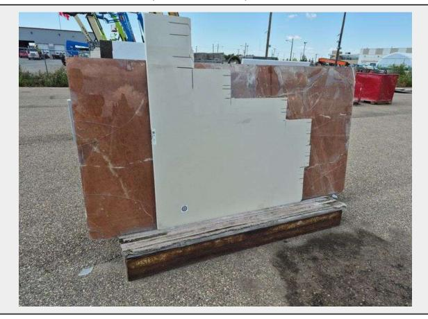
**Notes** 2 Slabs of Granite of Different Shapes, Sizes, and Colors, Glass Finish on 1 is cracking in several Places. Refer to Pictures
