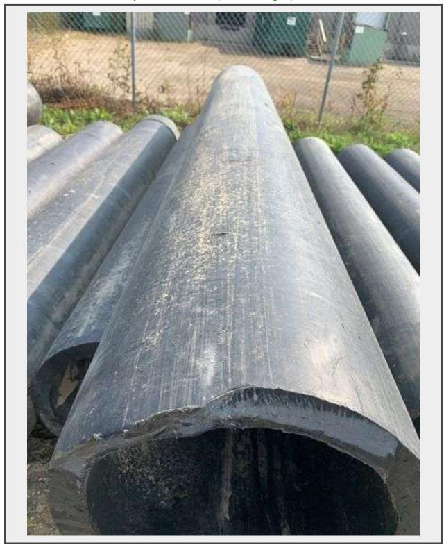
**Notes** PVC Sewer Pipe 20" Diameter, 12'2" Length, 2" Thick **Location** Edmonton
