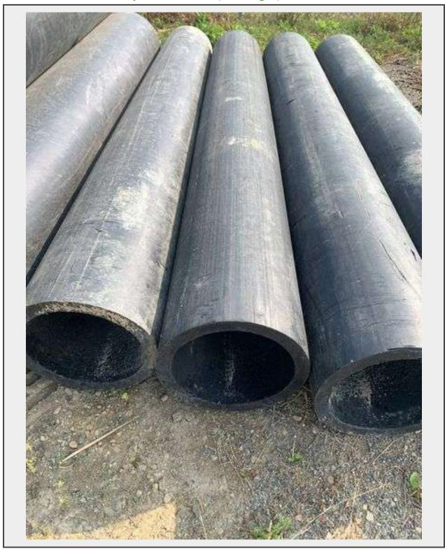
Notes PVC Sewer Pipe 16" Diameter, 10'Length, 1.5" Thick Location Edmonton
